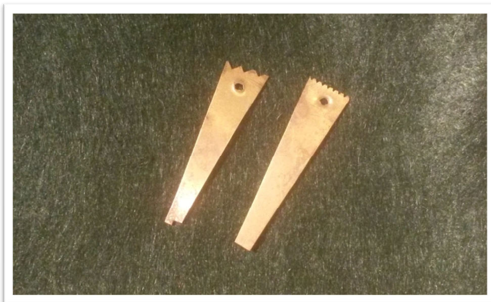
Figure 16 Samples of tabs cut on aiglet blanks
