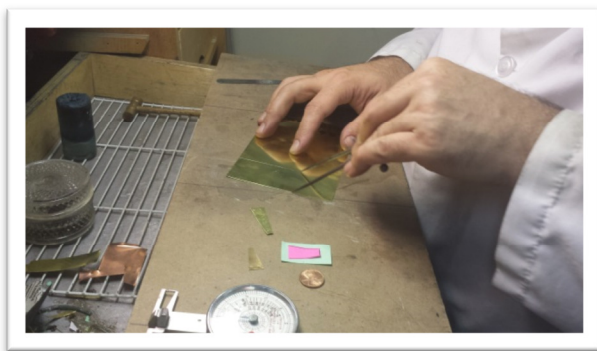
Figure 14 Scribing lines on brass sheet
