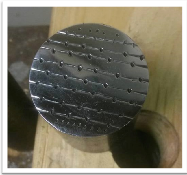
Figure 12 One inch die for imprinting aiglet blanks
