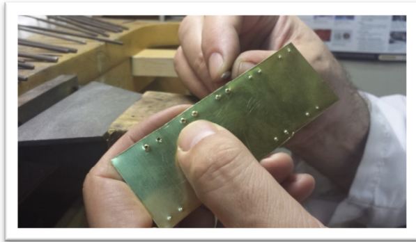
Figure 15 Back of the strip the blanks will be cut from showing the dimples left by the punch
