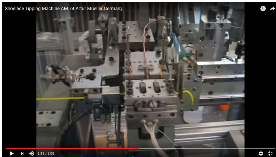
Figure 39: A Fully Automatic Lace Tipping Machine
