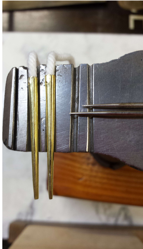
Figure 58: An assembled point ready to be riveted
