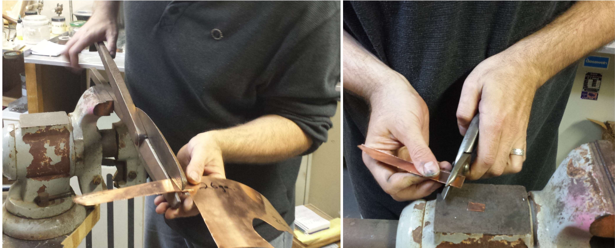
Figure 47: Cutting aiglet blanks with bench mounted and handheld shears
