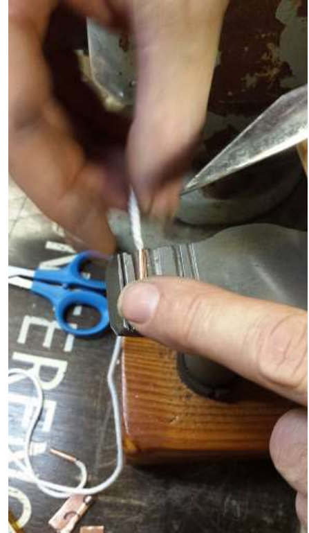
Figure 55: Manufacturing type 3 Aiglets, 3
