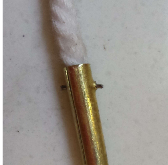
Figure 59: The iron wire inserted ready to be trimmed to length
