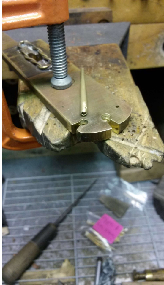
Figure 63: Tool for compressing the ends of aiglets
