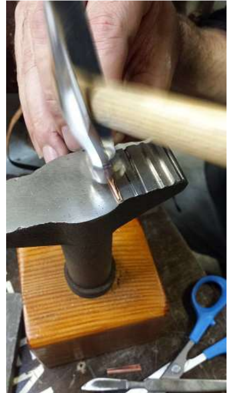
Figure 51: Manufacturing type 2 Aiglets, 3
