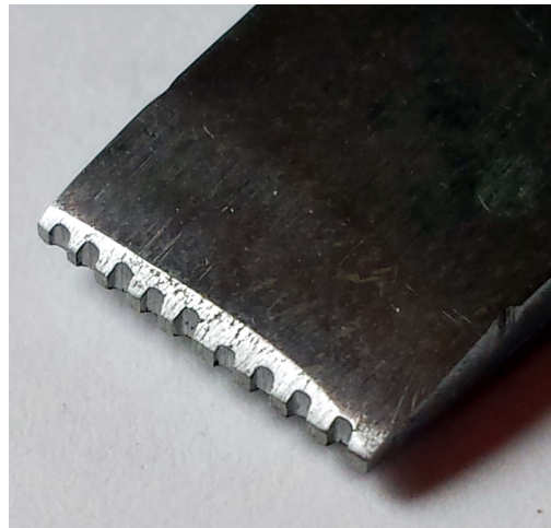
Figure 91: A punch to emboss a line of 10 square dots on aiglet blanks
