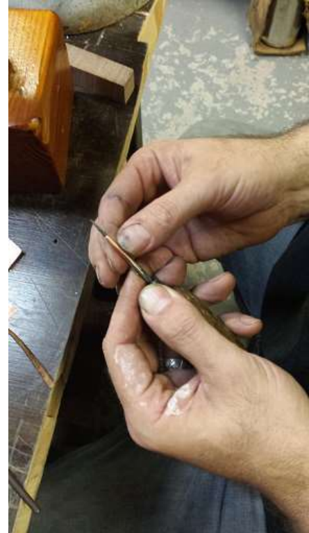
Figure 49: Type 2 aiglet, forming the blank around a mandrel
