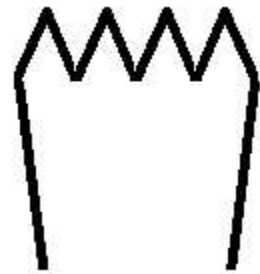
Figure 46: Cut tabs at the top end of the aiglet blank
