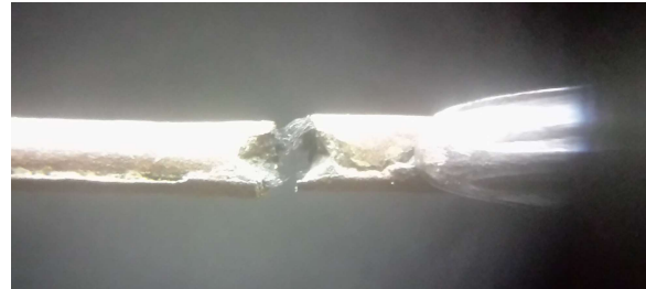
Figure 92: Thames Aiglet #18, detail of broken area
